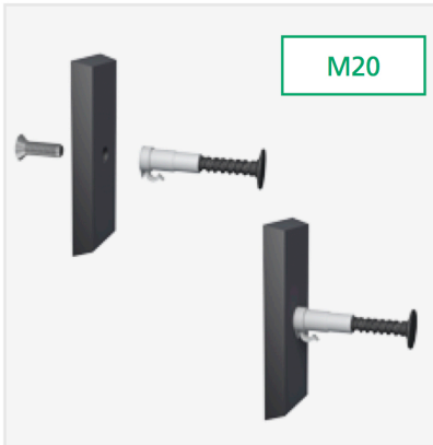
Attach the anchor sleeve to the Multibloc assembly element in accordance with structural requirements.
