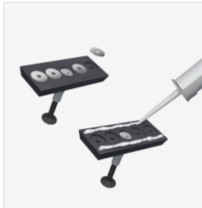
Secure the Multibloc to the formwork using magnets or hot-melt adhesive.
