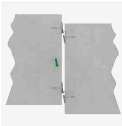
Stagger the wall elements on the building site in accordance with the assembly plan.
